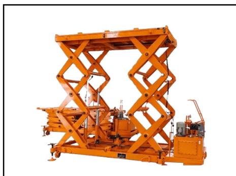
Representative image: Self-Elevating Platform used during EMCCR work in a PHWR maintenance environment
