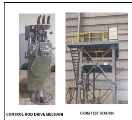
Representative image: Control Rod Drive Mechanism and test station used for reactor-control applications.
